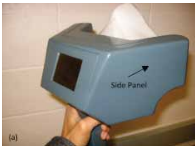
Figure 2: (a) RTM Upright View (b) RTM (side view) in operation for Alpha Detection
